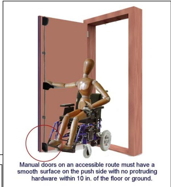
The design at the left is sort of hidden in the 2009 ANSI. It is the result of combining two of the ANSI requirements. It only applies to Type A Units in apartment complexes.
